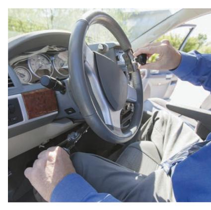
For an individual who has difficulty operating a car using a standard steering wheel and foot pedals, hand controls may be installed. Shown above is a steering wheel knob on the right and a lever for accelerating and braking on the left.
